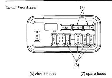
1. To check or replace a circuit fuse (6), pull the old fuse out of its retaining clips.
