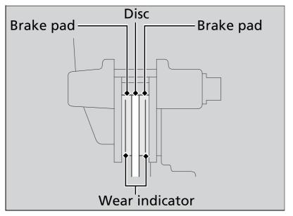
Inspect the brake pads from below the brake caliper.
