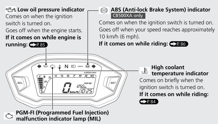
Comes on briefly when the ignition switch is turned on with the engine stop switch in the  $\bigcirc$  (Run) position. Comes on when the ignition switch is turned on with the engine stop switch in the  $\bigotimes$  (Off) position.
