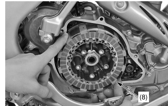
(8) clutch discs, clutch plates, judder spring and spring seat
