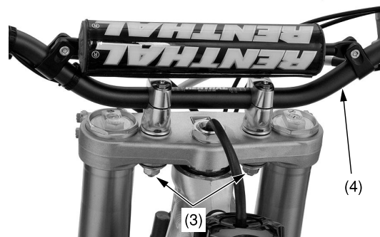
(3) handlebar lower holder nuts, washers and mounting rubbers (4) handlebar
