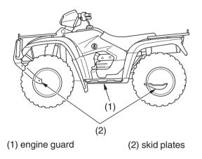
The engine guard (1) protects the engine crankcase. The skid plates (2) protect the frame and rear final gear case. Check the guard and plates for cracks, damage or looseness at intervals shown in the Maintenance Schedule.
