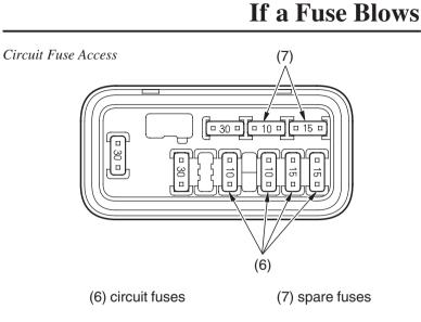
1. To check or replace a circuit fuse (6), pull the old fuse out of its retaining clips.
