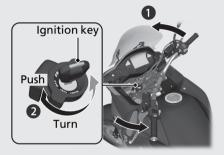
ON Turns electrical system on for starting/riding.
