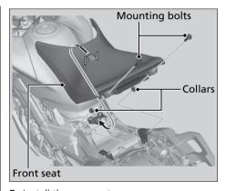
**5.** Install the rear seat. Make sure that the seat is locked securely in position to pull it up lightly.
