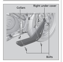
The right under cover must be removed to replace the engine oil filter.
