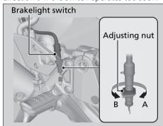
Brakes/Clutch ► Adjusting the Brakelight Switch
