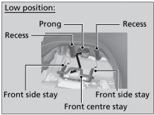
**6.** Make sure that the mount positions of the front seat prong and the adjust plates are the same seat position.
