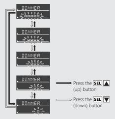
2 Press the **MODE** button. The backlight is set, and then the display moves to the changing of the speed and mileage unit.
