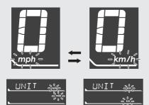
Press the MODE button. The speed and mileage unit is set, and then the display moves to the changing of the temperature gauge unit.
