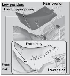
2. When setting the high seat position: Insert the front lower prong into the front stay.
