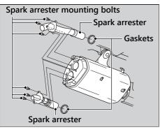
Use a brush to remove carbon deposits from the spark arrester screen. Be careful to avoid damaging the spark arrester screen. The spark arrester must be free of breaks and holes. Replace, if necessary. Check the gasket. Replace, if necessary.
