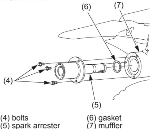
4. Remove the bolts (4), the spark arrestor (5), and the gasket (6) from the muffler (7).
