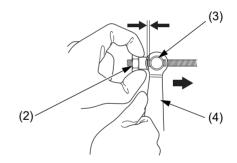
(2) adjusting nut (3) brake arm pin
