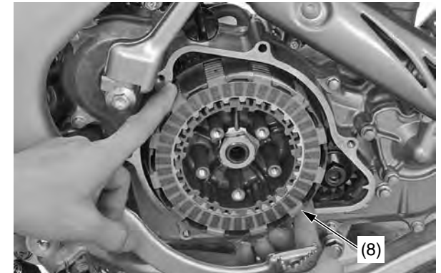
(8) clutch discs, clutch plates, judder spring and spring seat
