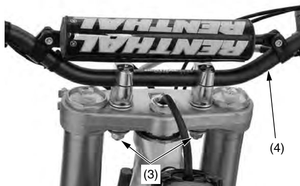
(3) handlebar lower holder nuts, washers and mounting rubbers (4) handlebar
