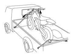
To secure your CRF, brace the front wheel against the front of the truck bed or trailer rail. Attach the lower ends of two straps to the tie-down hooks on your CRF. Attach the upper ends of the straps to the handlebar (one on the right side, the other on the left), close to the fork.
