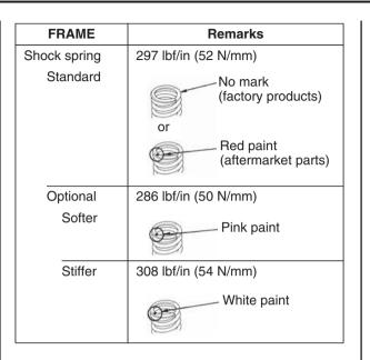
The standard shock spring mounted on the motorcycle when it leaves the factory are not marked. Before replacing the springs, be sure to mark them so they can be distinguished other optional springs.
