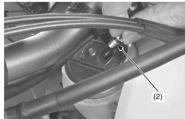
(2) pressure release screw
