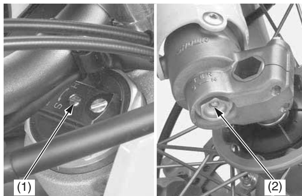
(1) compression damping adjuster screw (2) rebound damping adjuster screw
