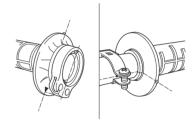
For added security, you may choose to bind the handgrips to the handlebar and throttle pipe with safety wires to prevent the possibility of them loosening. Position the twisted wire ends away from your palms and be sure to bend the wire ends well into the handgrip rubber so they will not snag your glove.
