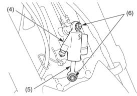
(4) steering damper(5) damper rod(6) steering damper mounting bolts
