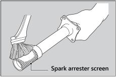
Install the gasket and the spark arrester, and tighten the spark arrester mounting bolts.
