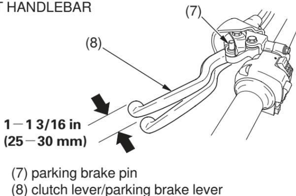
Check the clutch lever/parking brake lever and parking brake cable for loose connections or other damages. If the parking brake cable is worn or kinked, have it replaced by your dealer.
