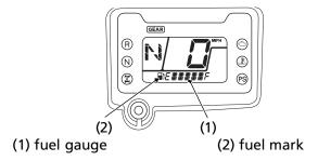
Regardless of what mode the display is in, when the fuel level reaches 1st segment (3), the display will automatically switch to the fuel gauge display. You should refuel as soon as possible. The amount of fuel remaining when the fuel gauge reaches the 1st
