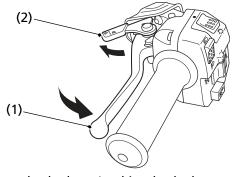
(1) rear brake lever/parking brake lever (2) P/R lever
