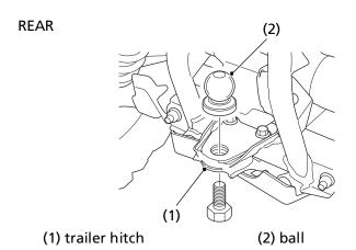
The trailer hitch (1) is located on the rear frame. To use the hitch, you'll need a proper size ball (2) as specified by the trailer manufacturer.
