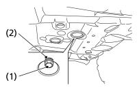
(1) engine oil drain bolt
