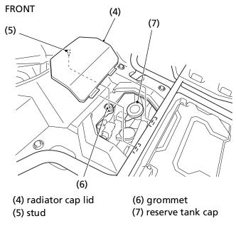
6. After adding coolant, reinstall the reserve tank cap. 7. Install the radiator cap lid.
