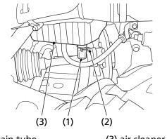
(1) drain tube(3) air cleaner housing(2) clip
