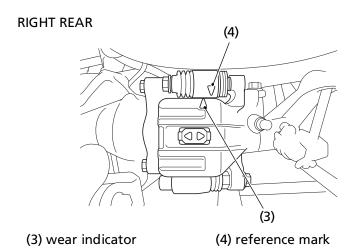
Check the wear indicator. If the wear indicator (3) aligns with the reference mark (4), replace both pads as a set, see your dealer for this service.
