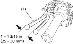
(1) rear brake lever/parking brake lever
