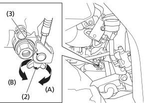
(2) brake lever adjusting nut(3) brake arm pin
