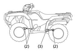
(2) rubber propeller shaft boots
