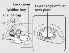
Do not fill with fuel above the lower edge of the filler neck plate.
