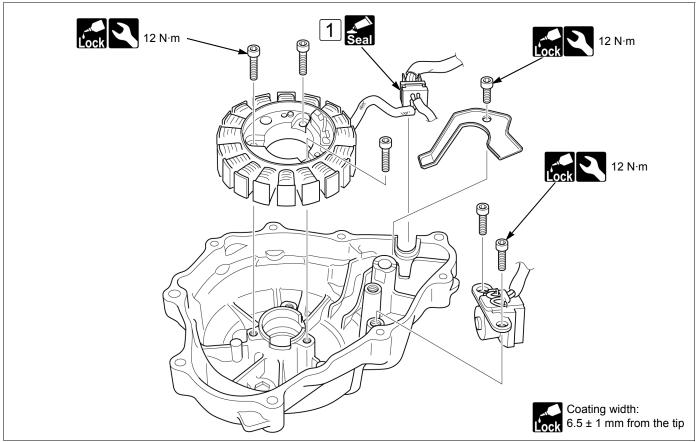
• 1 Apply sealant (TB 1141G, 1215, 1207B, or equivalent) to the sealing surface.
