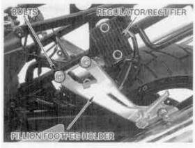
Remove the seat rail mounting bolts, nuts and seat rail.
