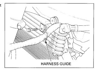
Install and tighten the oil cooler upper mounting bolts.
