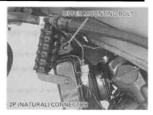
Install the main wire harness guide onto the left mounting boss as shown.
