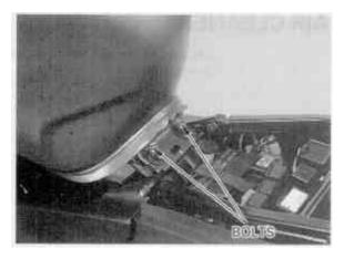
Support the front end of the fuel tank using a suitable support as shown.
