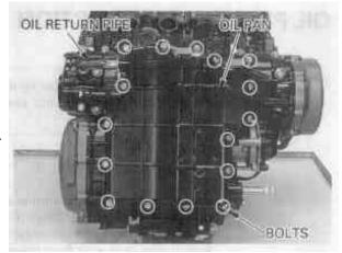
Remove the bolt and oil return pipe bracket. Remove the oil return pipe and O-rings.
