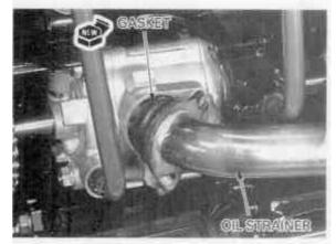
Install the oil strainer set plate aligning its cut-outs with the oil pipes.
