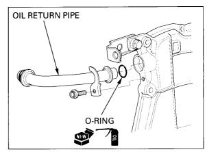
Install the set plate and tighten the bolt to the specified torque.
