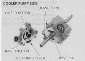
Remove the oil pump spacer and dowel pins.
