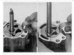
Measure the side clearance for the feed and cooler pump using a straight edge and feeler gauge.
