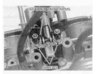
Loosen the lock nuts and remove the starter valve assembly.
