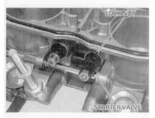
Clean the starter valve bypass using compressed air.
