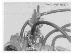
Remove the starter valve arm screws and starter valve arms.
