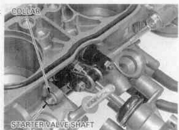
Install the starter valve assembly into the valve hole.
