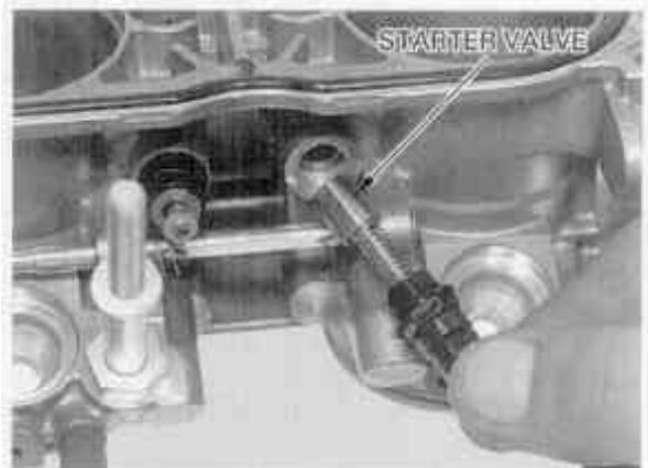
Tighten the starter valve lock nut to the specified torque.
